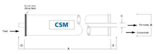
Each membrane element supplied with one brine seal, one interconnector (coupler) and four o-rings.
